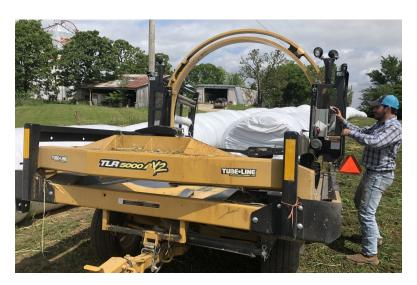
Baling corn wet and then tubing the bales in plastic wrap is a good way to handle this feed. It captures enough moisture that the bales will ensile in the tube, nitrate levels will drop, and the stalks become more palatable for livestock. Baling this product between 50 - 60% moisture will help capture the best feed value and ensure the ensiling process.
